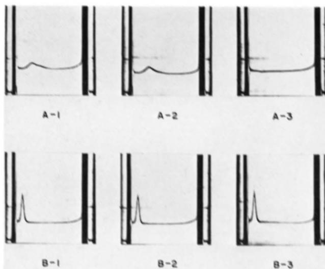
FIG. 7. Effect of prior treatment of LDL with phospholipase A on the sedimentation behavior of DS-LDL mixtures and LDL sample alone. LDL samples were treated with phospholipase A in the usual manner. Samples 1 and 2 are the treated LDL in which 29 and 94%, respectively, of the phosphoglyceride constituents were hydrolyzed; sample 3 is control LDL. A, sedimentation patterns of 0.0075% DS-0.25% LDL mixture; B, 0.25% LDL alone. The photographs were taken 14 min after reaching the maximum speed.
